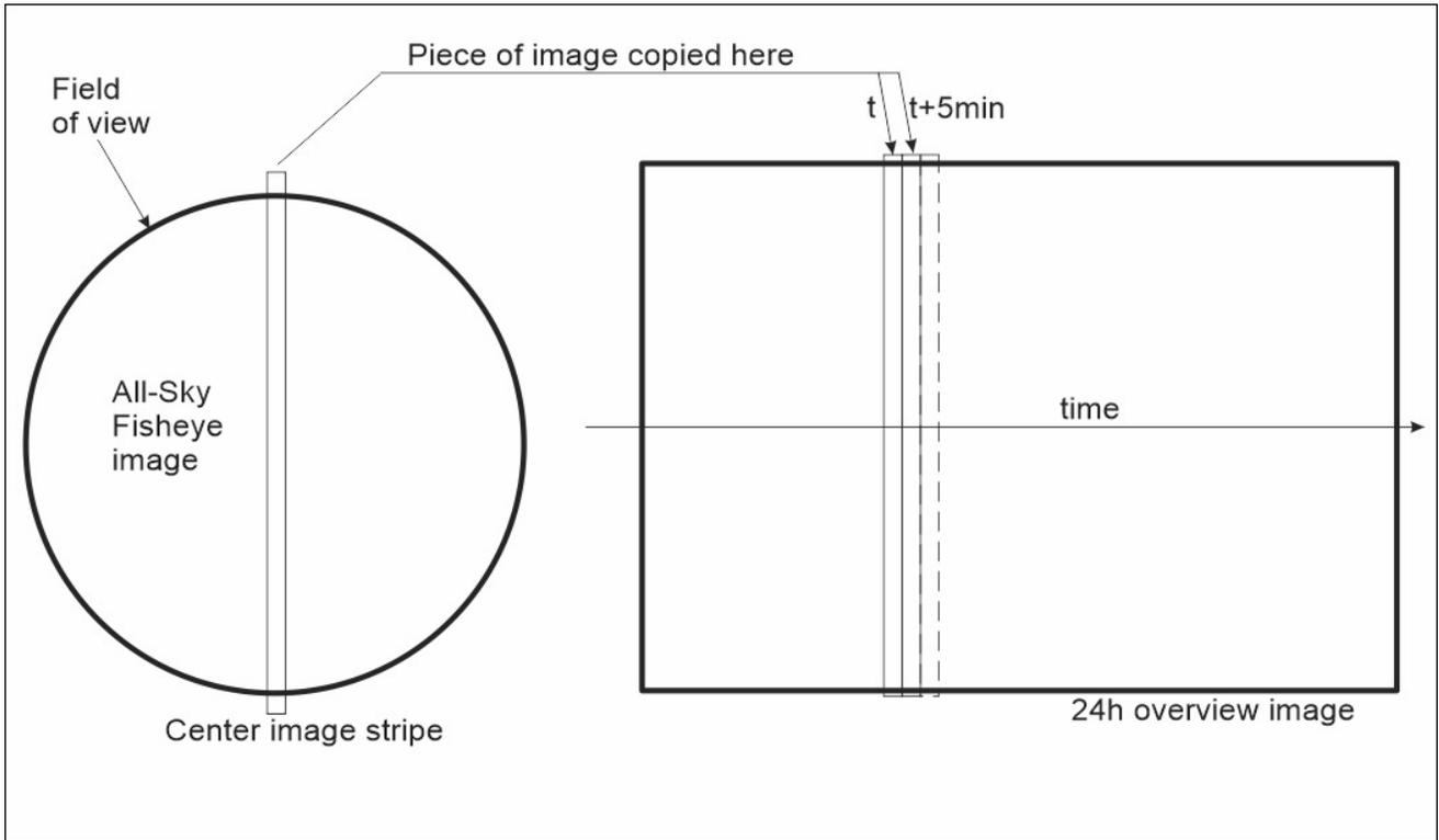
Fig. 58 : 24h image overview construction scheme
