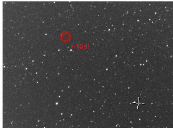
Fig. 55 Telescope position as red because current date and telescope position date is larger than 10s
