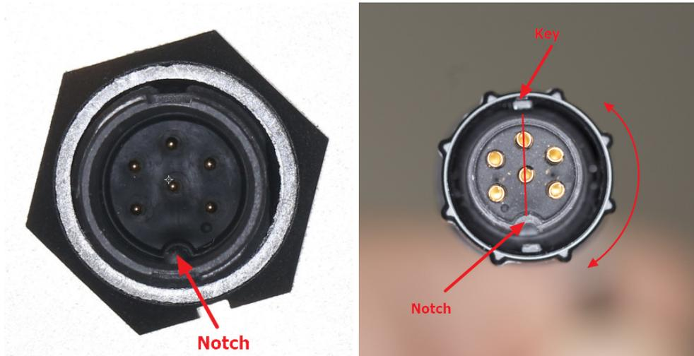
Fig. 4 Left, camera panel connector, right cable connector, please align key to the notch prior attaching the connector to the camera.
