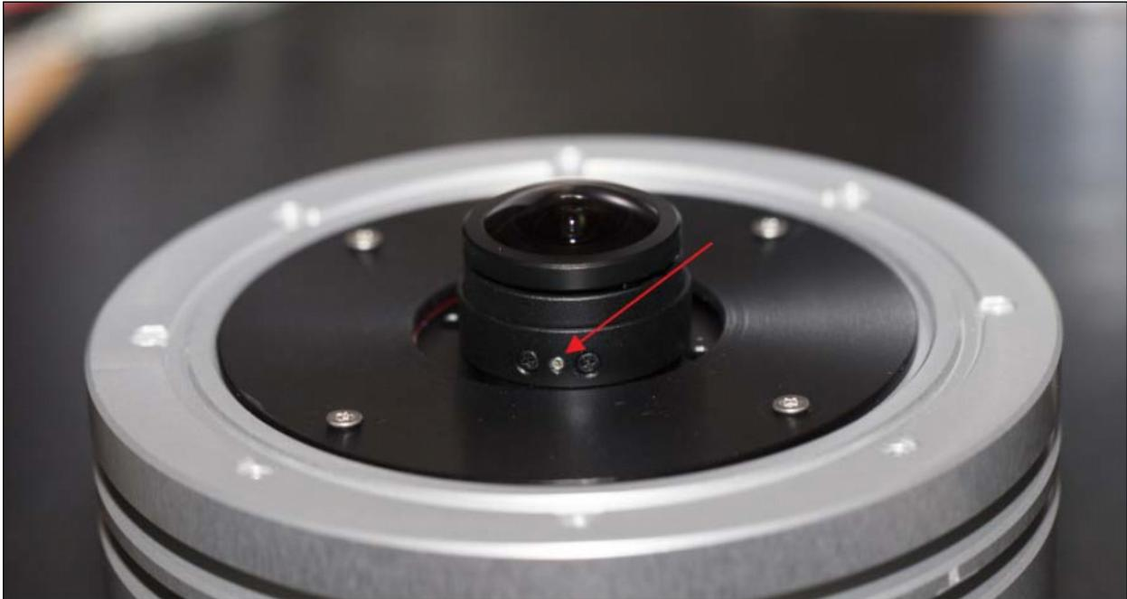
Fig. 64 ALPHEA 3xx camera, the small cap screw to lock/unlock the focus.
