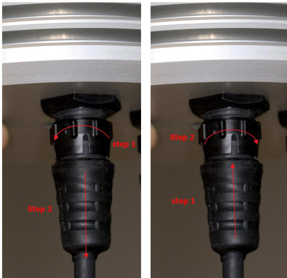
Fig. 5 Steps to detach (left) and attach (right) the cable connector to the camera
