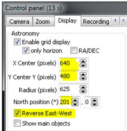
Fig. 47 displacement in X and Y to adjust the position of the zenith symbol
