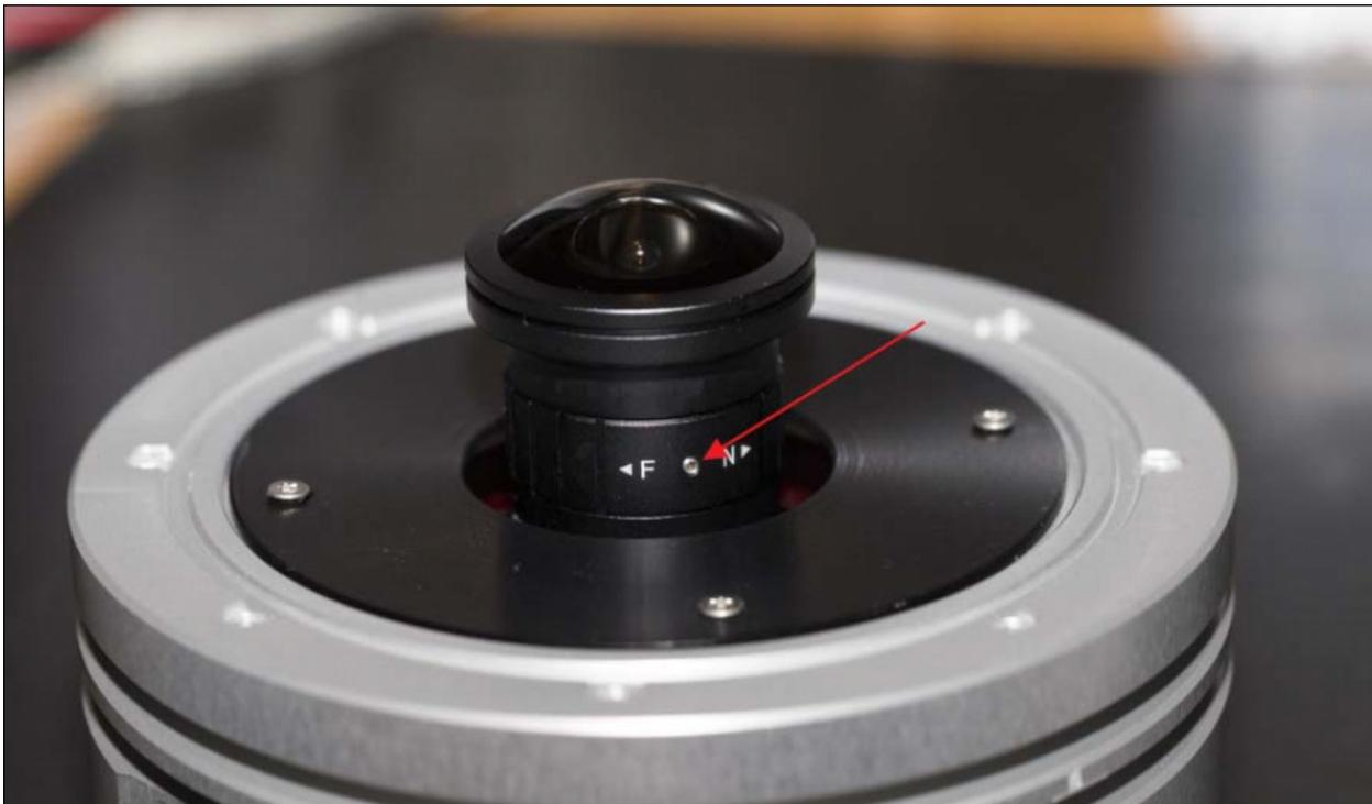
Fig. 63 ALPHEA 6xx camera, the small cap screw to lock/unlock the focus
