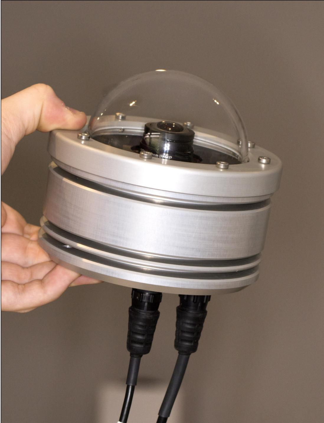
Fig. 3 *USB and power cable connected to the camera.*
