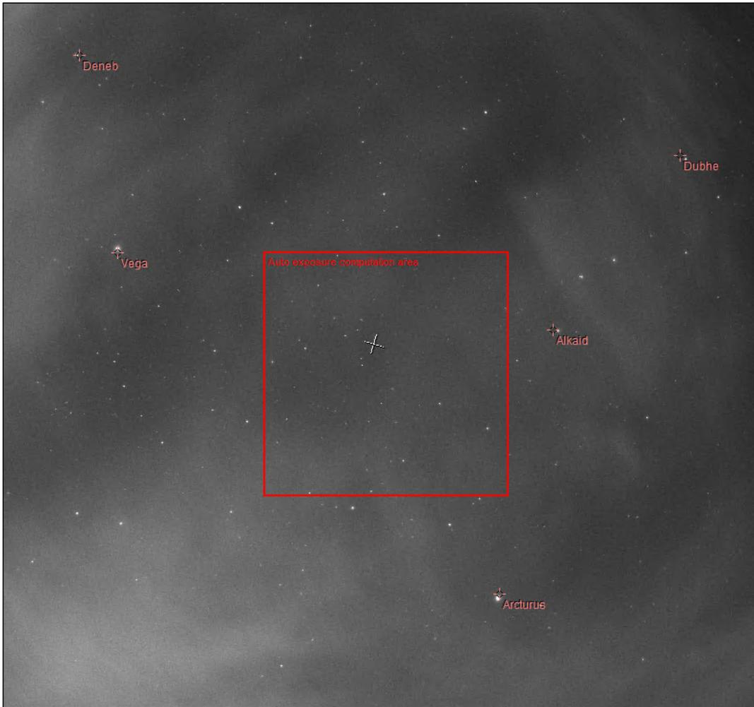
Fig. 28 If the computing area for auto exposure is set to 512x512 image center, this shape is drawn to show where the bounds of this area are located.
