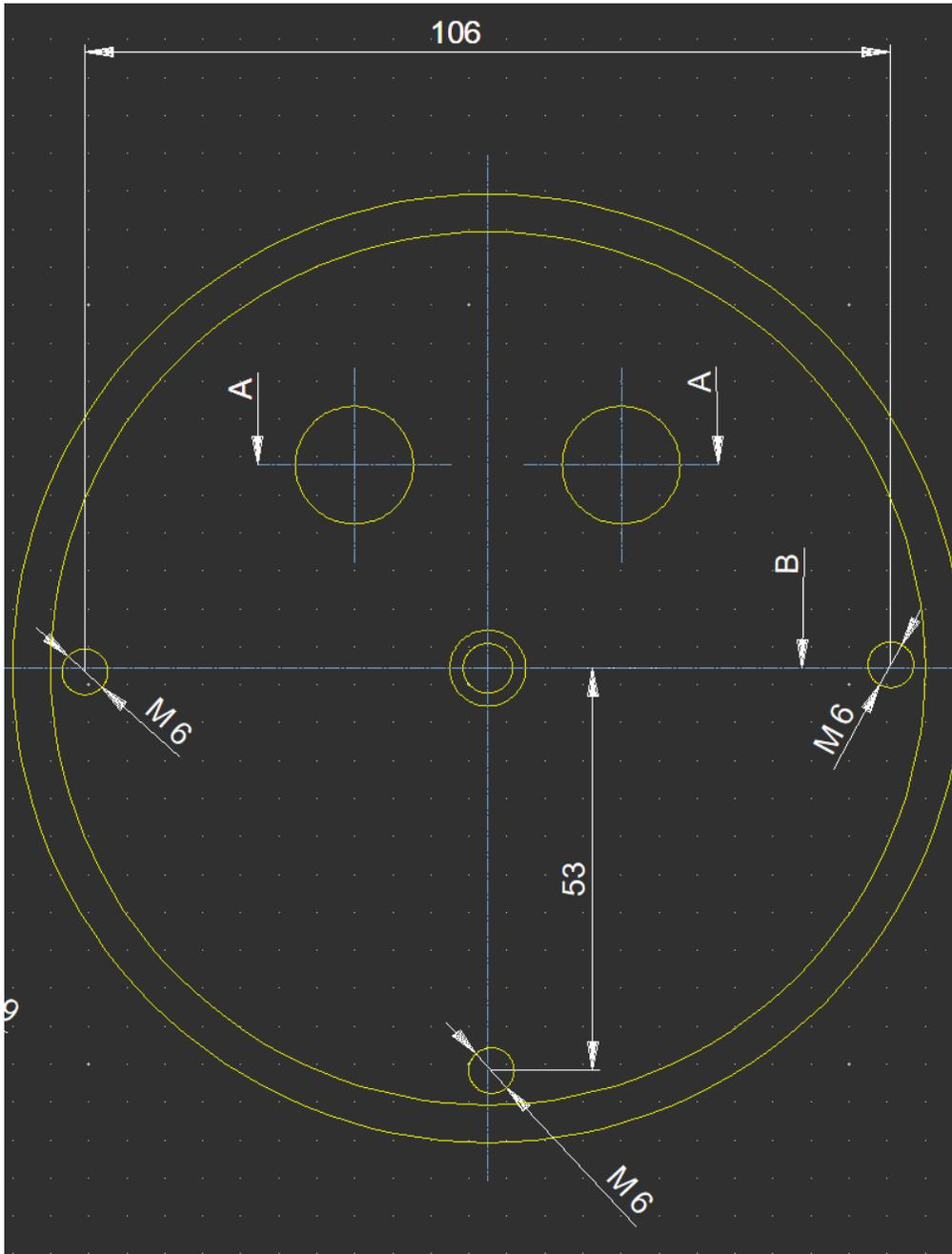
Fig. 2 The position of the three M6 screws underneath the camera and the two connectors
