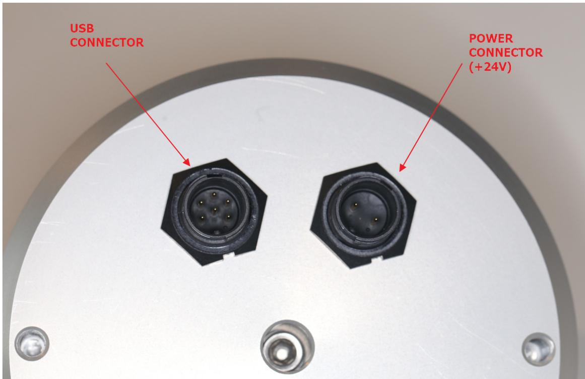
Fig. 6 Six pins connector when cable is detached from it.
